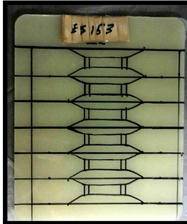
Figure 1: Prepared epoxy-silica nanocomposite (ES153) dog-bone specimens prior to tensile testing, conforming to ASTM D638 standard dimensions.
