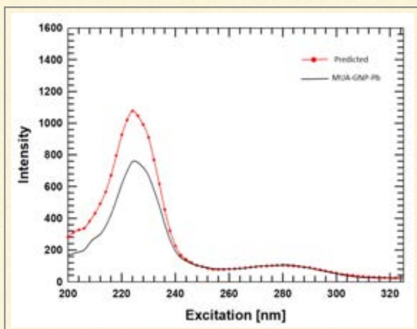
Figure 7. 2D spectrum of MUA-GNPs at 11.375 µg/mL with Pb<sup>2+</sup> at 100 µg/L
