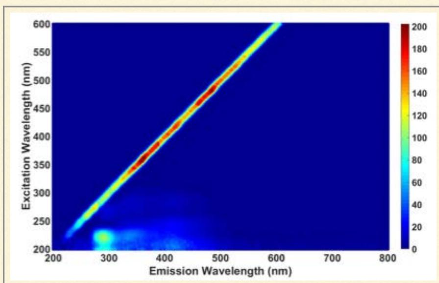
Figure 3. EEM spectrum of 100 µg/L Pb<sup>2+</sup> in HPLC grade water.
