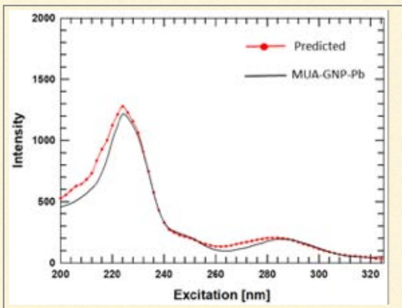
Figure 5. 2D spectrum of MUA-GNPs at 11.375 µg/mL with Pb<sup>2+</sup> at 100 µg/L
