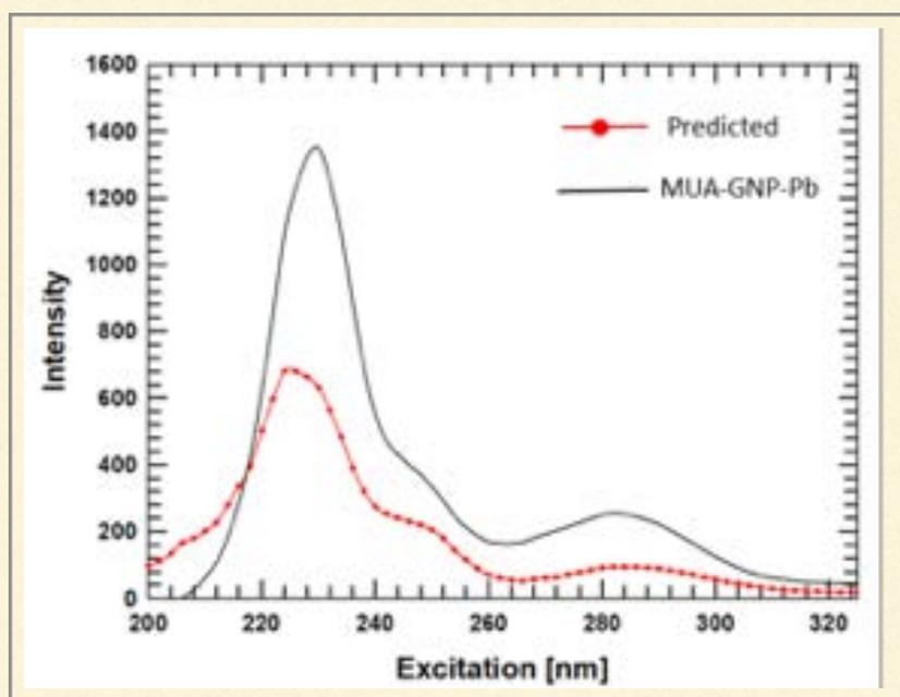
Figure 6. 2D spectrum of MUA-GNPs at 11.375 µg/mL with Pb<sup>2+</sup> at 100 µg/L
