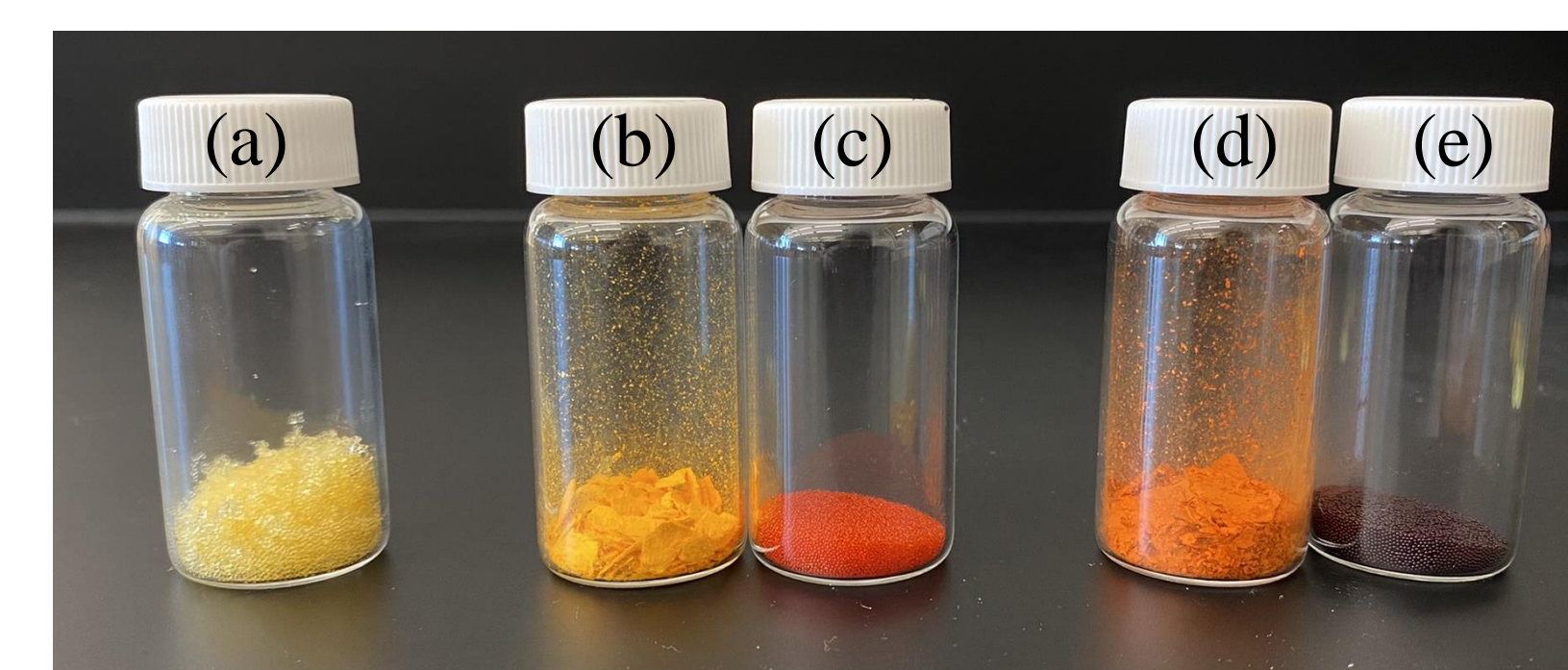
Figure 5: (a) Unmodified Resin, (b) NQSA-PSC Ligand, (c) NQSA-PSC Chelating Resin, (d) NQSA-PTSC Ligand, (e) NQSA-PTSC Chelating Resin
