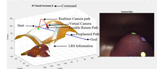
Fig. 6 Real-time Guidance System
