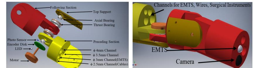
Fig. 4 Disassembly of Single Joint
