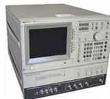
Fig. 3: An HP 4194A impedance analyzer
