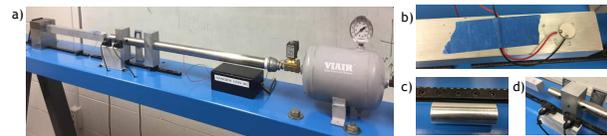
Fig. 6: (a) Experimental system, (b) Incident beam with PZT, (c) Striker bar, (d) Velocity sensors
