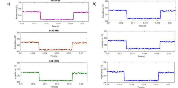
Fig. 9: Impedance results for incident beam impacted at 2.09 m/s, while being excited with (a) individual single-tone excitation signals, (b) Multi-tonal excitation signal
