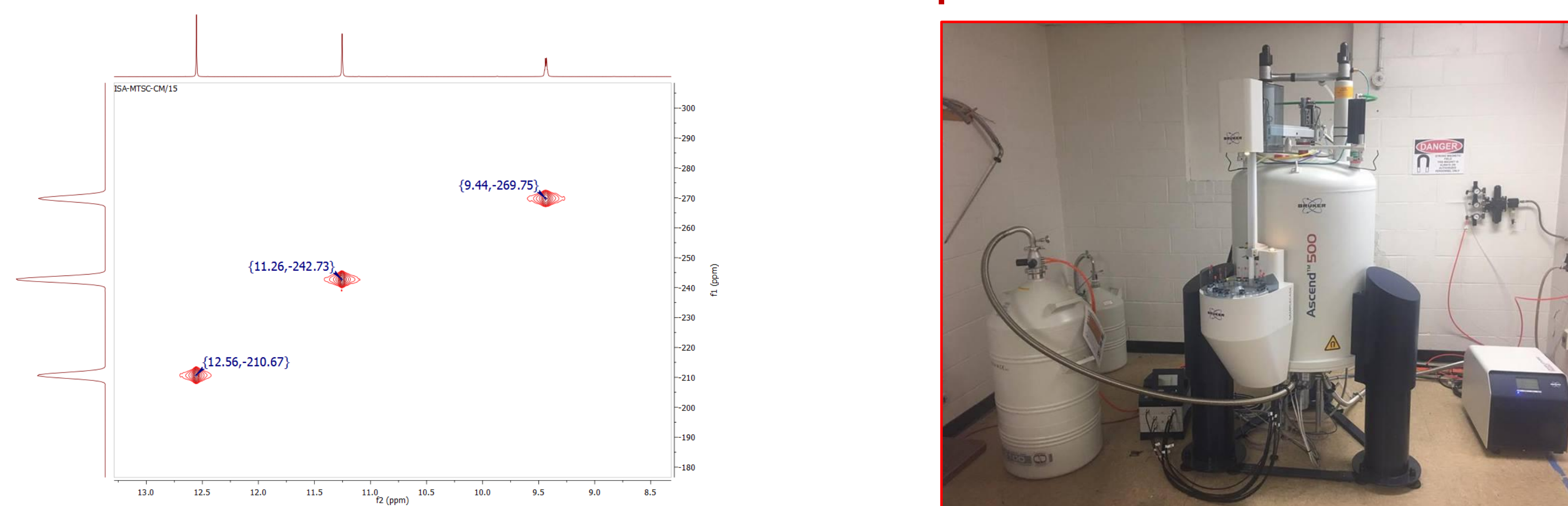
Figure 3. The 2-D 1 H, 15 N Heteronuclear Single Quantum Coherence NMR Spectrum of ISA-MTSC obtained on Bruker Ascend-500 Multi-Nuclear NMR Spectrometer
