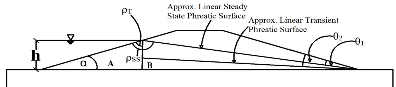
**Figure 5. Variables used in deriving standardized equations, T and S**
