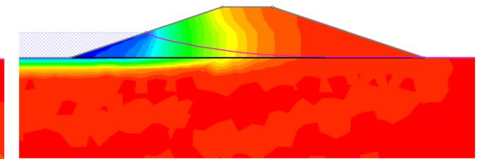
**Figure 4b. Transient seepage results for silt-like levee on clay-like foundation**
