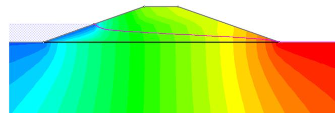
**Figure 4a. Transient seepage results for silt-like levee on sand-like foundation**
