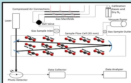
Figure 2: The schematic diagram of Cavity ring-down spectroscopy set-up and the associated components in the laboratory.
