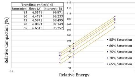
Figure 1A (top) Clay Soil Compaction Results
