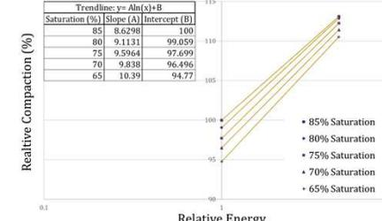
Figure 3A (top) Shale Compaction Results
