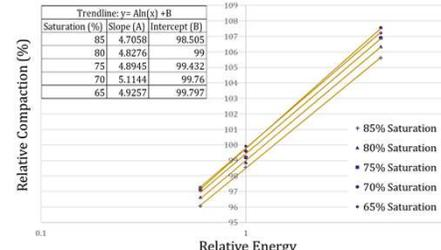
Figure 2A (top) Limestone Sand Compaction Results
