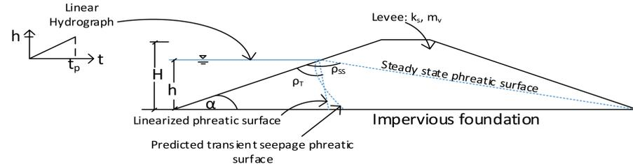
Fig 1. Idealized levee saturation after flood
