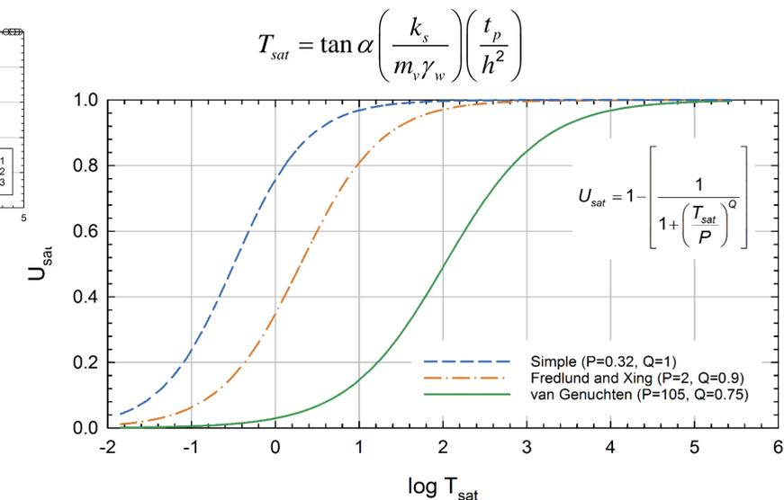
Fig 5. Comparison of hyperbolic curves for estimation of levee saturation
