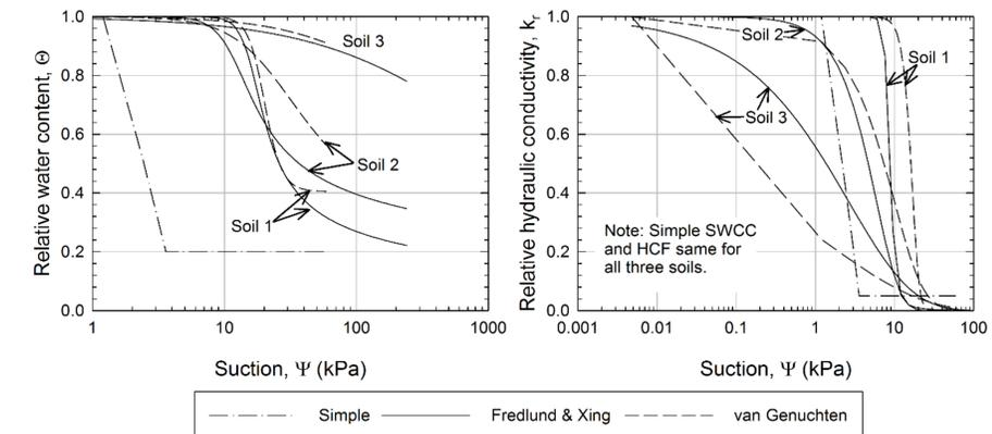
Fig 3. Comparison of Simple, Fredlund and Xing, and van Genuchten models SWCC and HCF models
