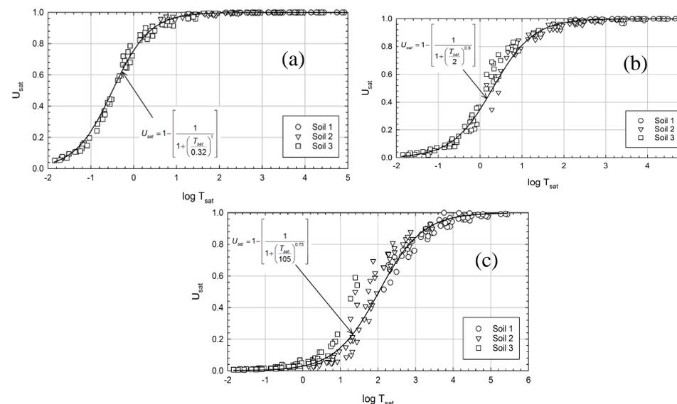
Fig 4. Extent of levee saturation predicted by a) Simple, b) Fredlund and Xing, and c) van Genuchten models
