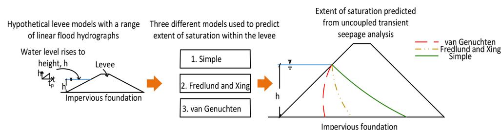
Fig 2. Methods used to predict extent of levee saturation using van Genuchten, Fredlund and Xing, and a Simple unsaturated soil model
