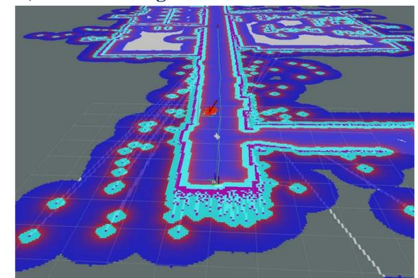
**Figure 3:** Cost map generated by Lidar and Ultrasonic Sensors, the map generated is used for obstacle detection. **Figure 4:** The green line indicates the path to be used by the wheelchair to get to its destination, and the red particles with the arrow indicates the actual position/path of the wheelchair
