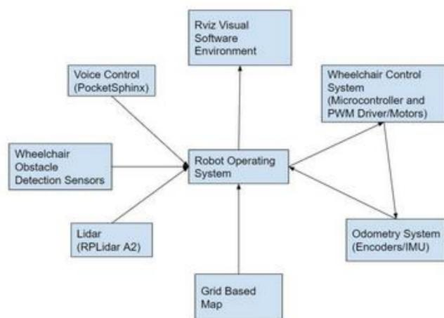
The Robot Operating System (ROS), is the framework used to write the robot's software. ROS Visualization (RVIZ) is the visualizer used along with ROS for displaying sensor data. It helps in easier representation and analysis of sensor data.
