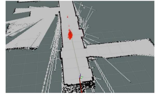
**Figure 1:** Map of the fourth floor of Brown Hall created with a LIDAR Sensor and Hector Mapping Algorithm. **Figure 2:** Localization of the wheel chair using the AMCL algorithm in the Map created.
