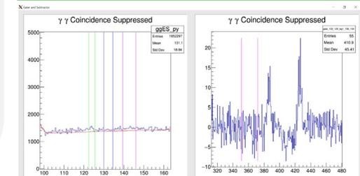
Figure 6: TBGSubtraction gated on 123 keV peak with 426.4 keV peak found in coincidence.
