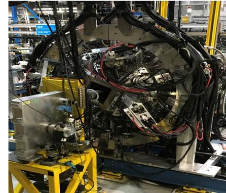
Figure 4: GRIFFIN array with moving tape collector on left.
