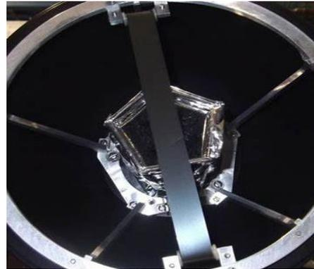
Figure 3: Moving tape collector inside GRIFFIN along with 5 of 11 SCEPTAR scintillators.
