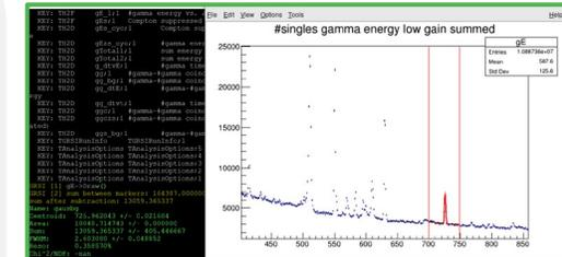
Figure 5: Fitting peaks via Gaussian curve with the GRSISort analysis tool.
