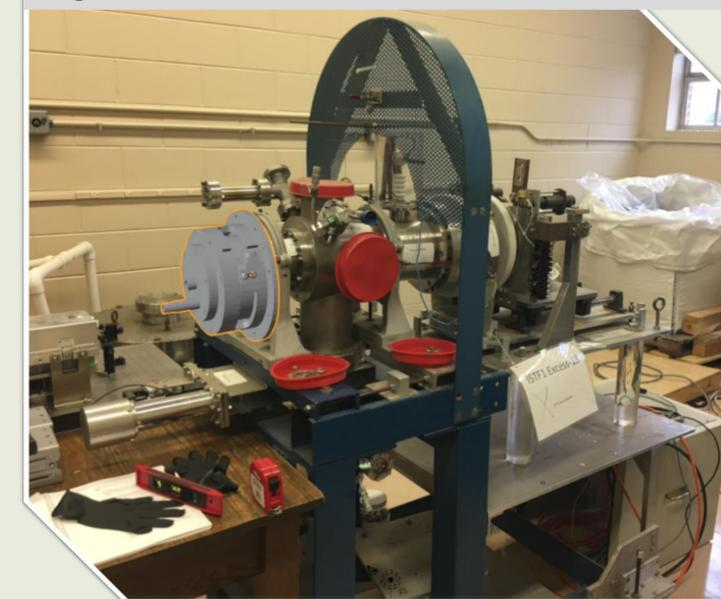
Figure 5: High Voltage Platform w/ Proposed Ion Generator in grey
