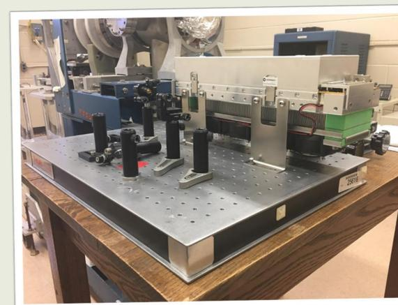
Figure 3: Optical Table & Laser
