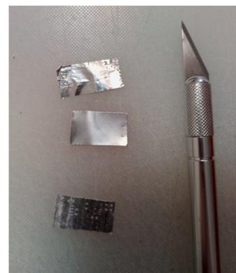
**Figure 4:** The can was much too thick to accurately cut the precise pieces with only a craft tool or boxcutter. Aluminum foil (top sheet) was then attempted to be cut out but was much too flimsy to withstand the multiple cuts and pressure without tearing.
