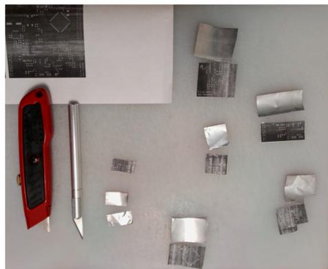
**Figure 3:** One attempt to help resolve the issues with the paste was utilizing a soda can to make a stencil. After three days of being unrolled and placed under three full bottles of wine, the can would still roll back up to its original shape. The can was cut into individual pieces that could be smoothed out before attempting to cut the tiny component pieces out.
