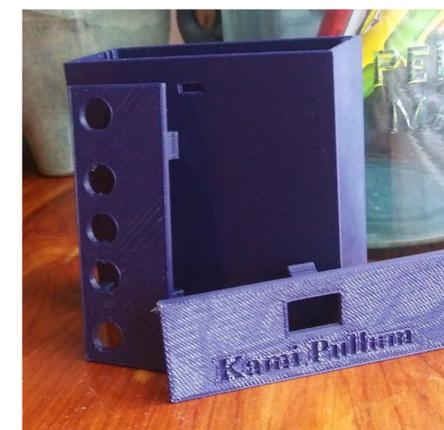
**Figure 7:** 3D Printed box for DStat potentiostat
