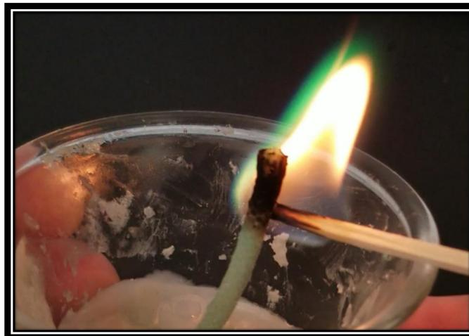
Figure 1. Copper (II) sulfate candle
