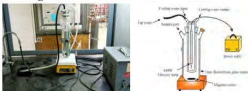
Fig. 4, & 5. TiO<sub>2</sub> thin film coating insert on UV Photocatalytic reactor using aluminum rods
