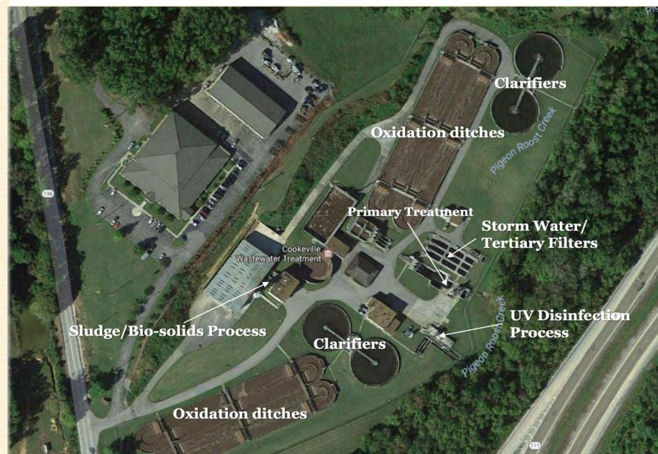
Fig. 3 : Aerial view of the layout of Cookeville WWTP (Reference [2])
