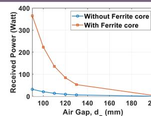
Figure 15: Transfer Power-With and Without MM
