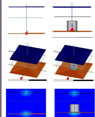
Figure 6: ANSYS based model with (right) and without (left) MM Ferrite core. Top- Front View, Middle-Side View Bottom- Distribution of H-field
