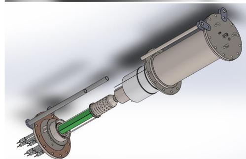
A Test stand structure to contain this vessel along with all of the control components, electronics, and gas plumbing was created. The vessel is surrounded in a nitrogen environment to ensure no combustion occurs inside the test stand enclosure. This structure allowed for the vessel to be oriented vertically to allow for the use of a crane to raise and lower the outer piping of the pressure vessel. The below figure displays the entire test stand.
