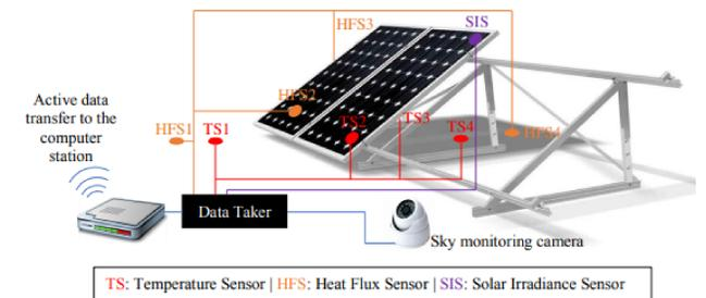
Experimental Setup to collect time-varying boundary conditions to feed the CFD simulations
