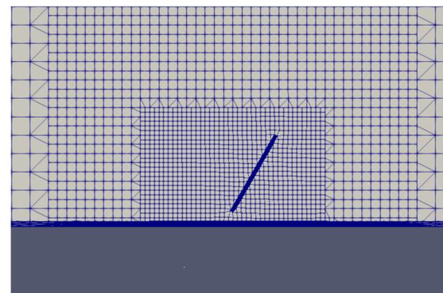
Mesh Cross Section Of A Single Panel Row
