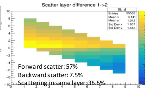
Figure 6: A plot showing the difference in segment between first and second scatter of 1MeV neutrons. In the bottom left corner are statistics produced with my root macro.
