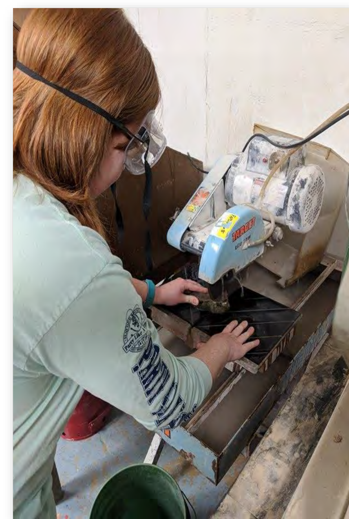
Figure 5. (Below) Cutting samples using a wet saw. Figure 6. (Right) Polishing the samples along the bedding plane.
