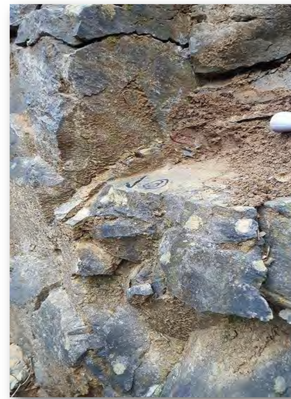
Figure 2. Oriented sample of the Bangor Limestone from Brown Gap Quarry, Sequatchie Valley.
