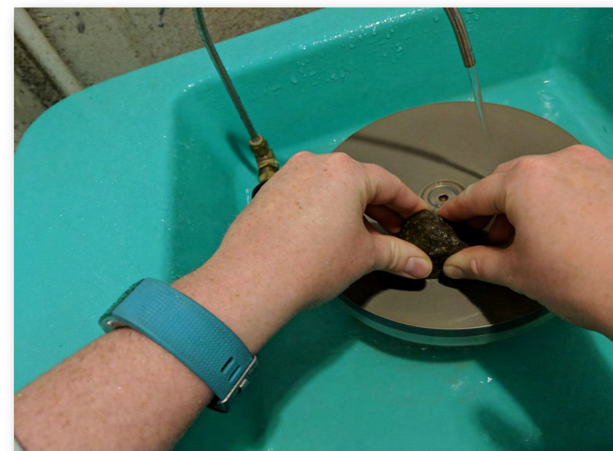
Figure 5. (Below) Cutting samples using a wet saw. Figure 6. (Right) Polishing the samples along the bedding plane.
