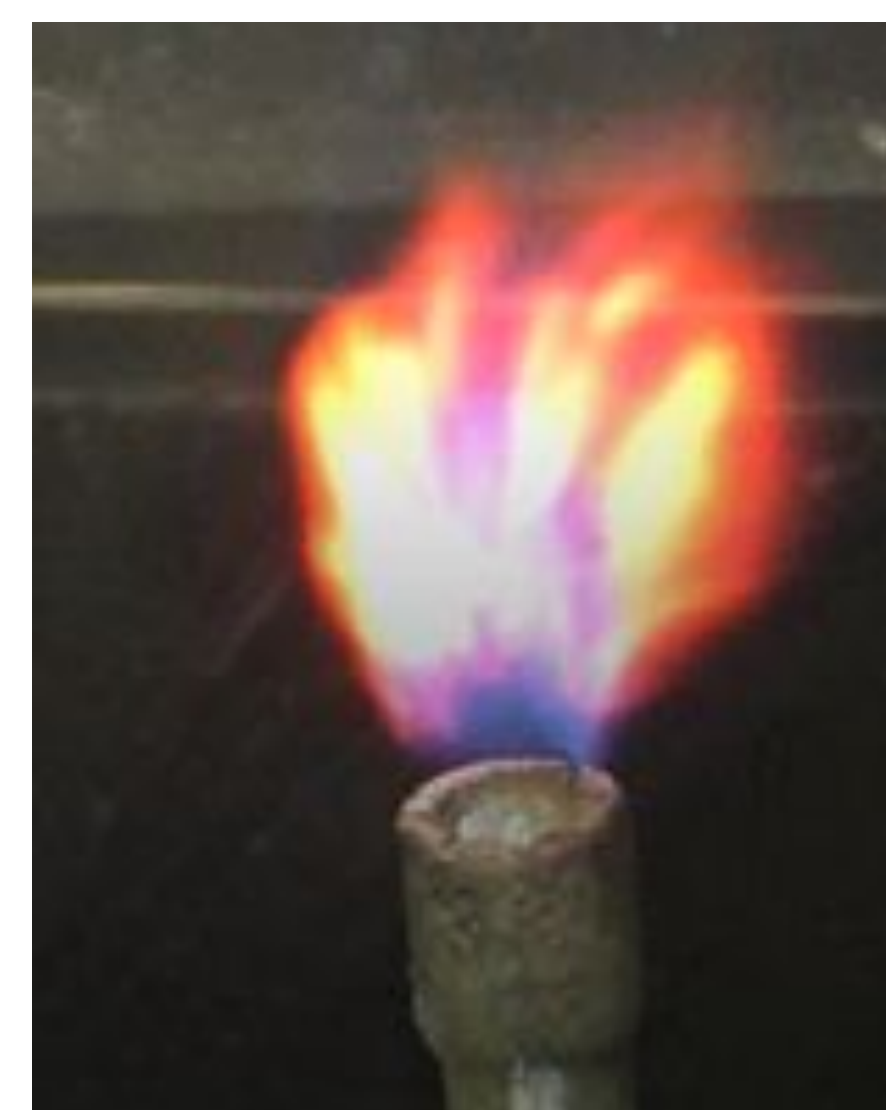
Figure 1: Strontium chloride flame by spray method
