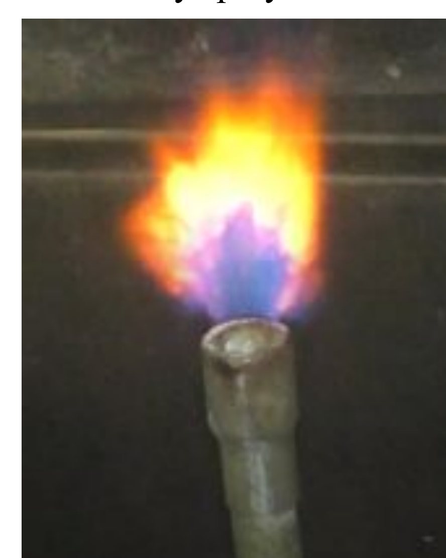
Figure 13: Calcium nitrate flame by spray method
