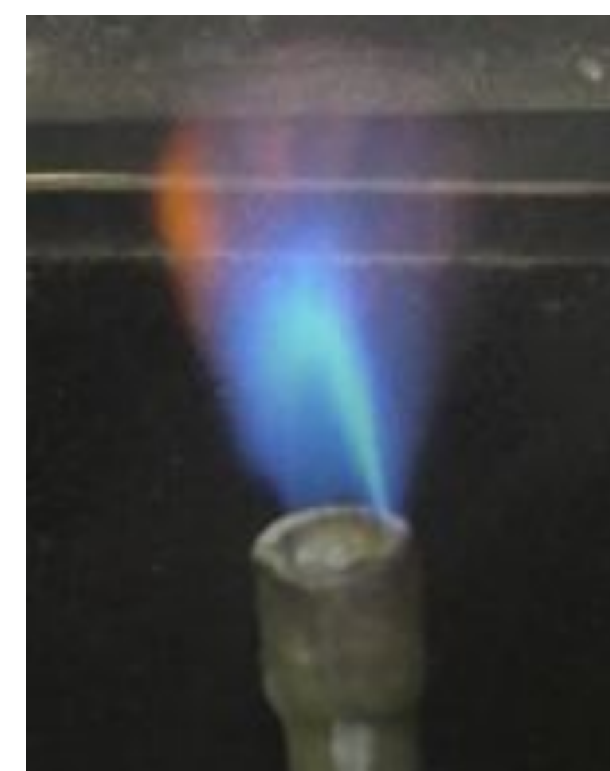
Figure 5: Magnesium sulfate flame by spray method
