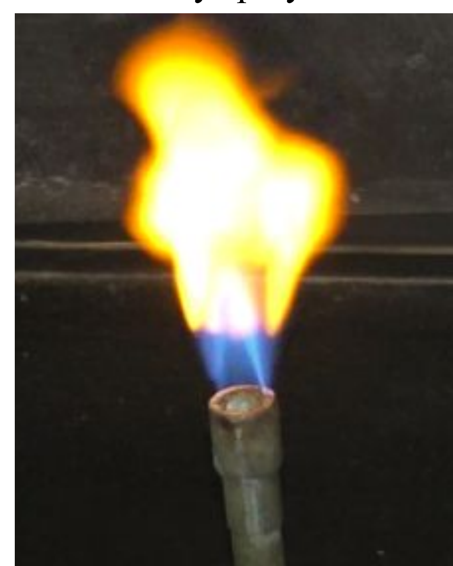
Figure 11: Sodium chloride flame by spray method
