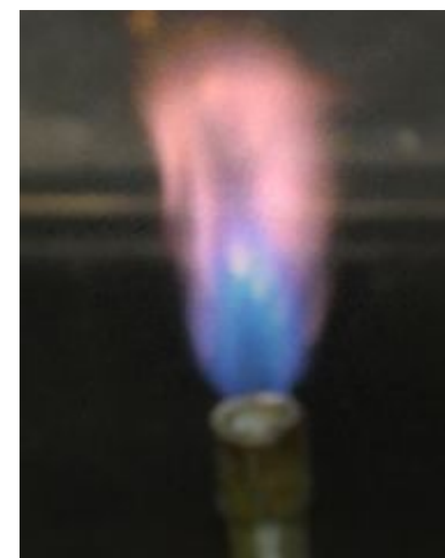
Figure 6: Potassium chloride flame by spray method
