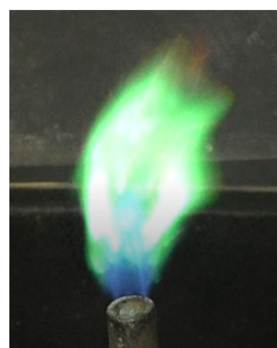
Figure 7: Copper (II) chloride flame by spray method
