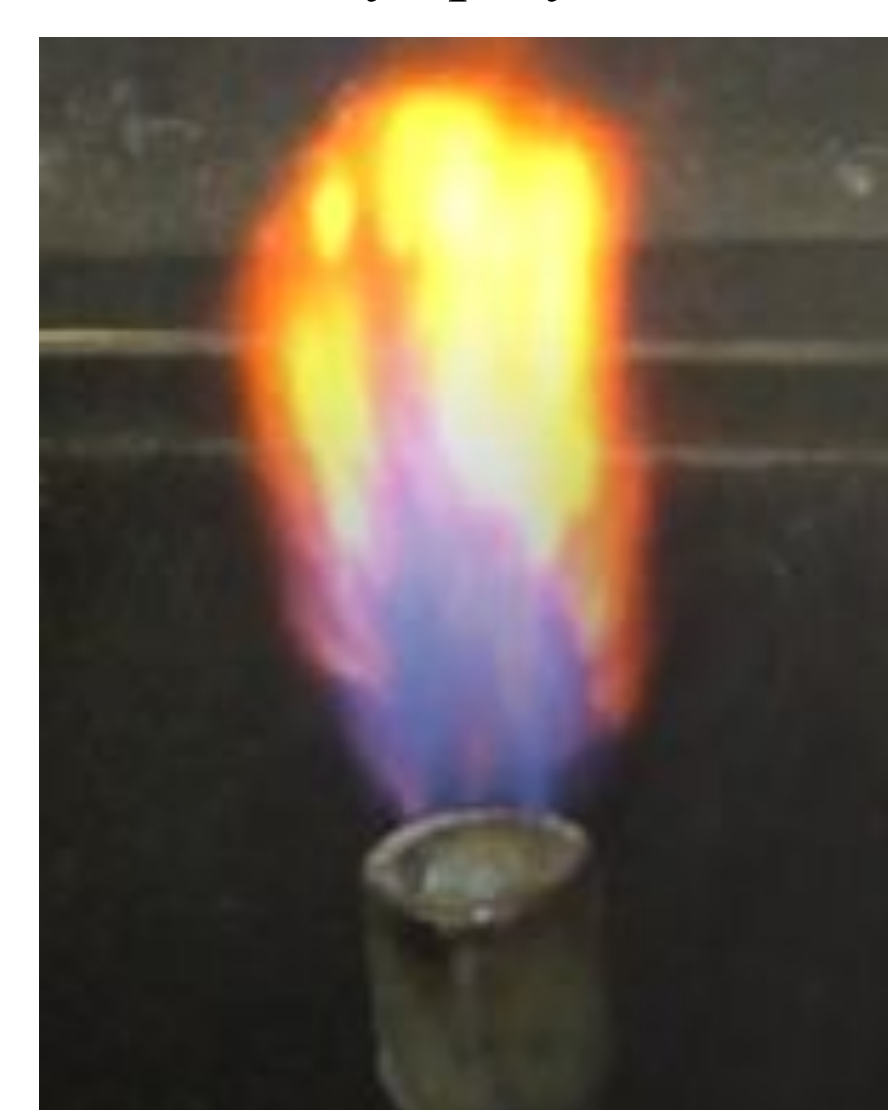
Figure 12: Calcium chloride flame by spray method
