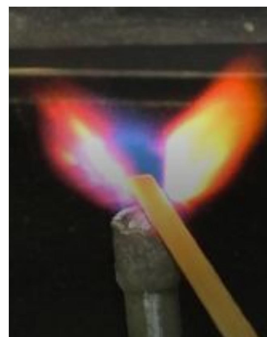
Figure 2: Strontium chloride flame by wooden stirrer method
