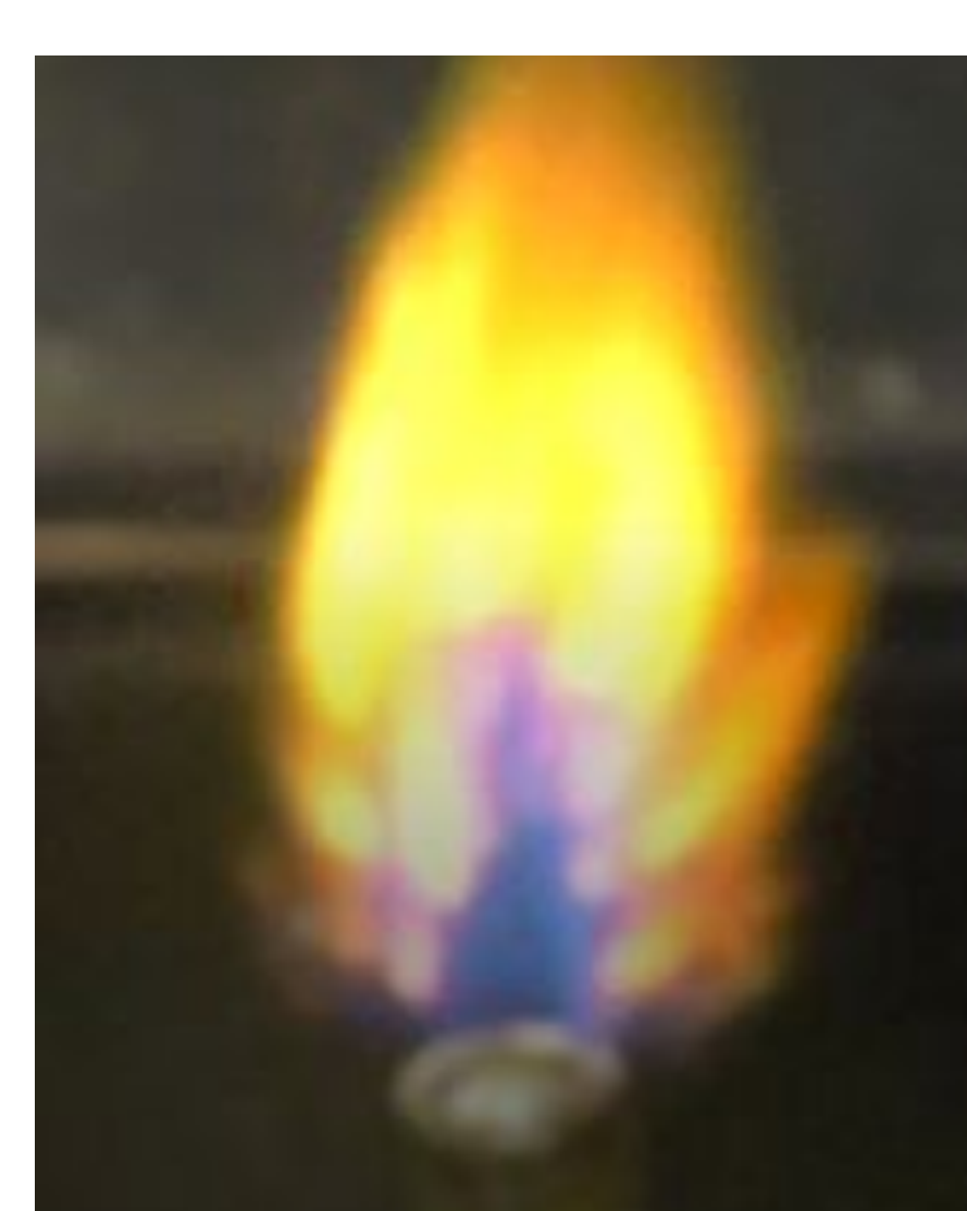
Figure 9: Barium chloride flame by spray method
