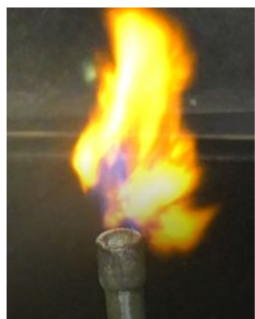
Figure 10: Borax solution flame by spray method
