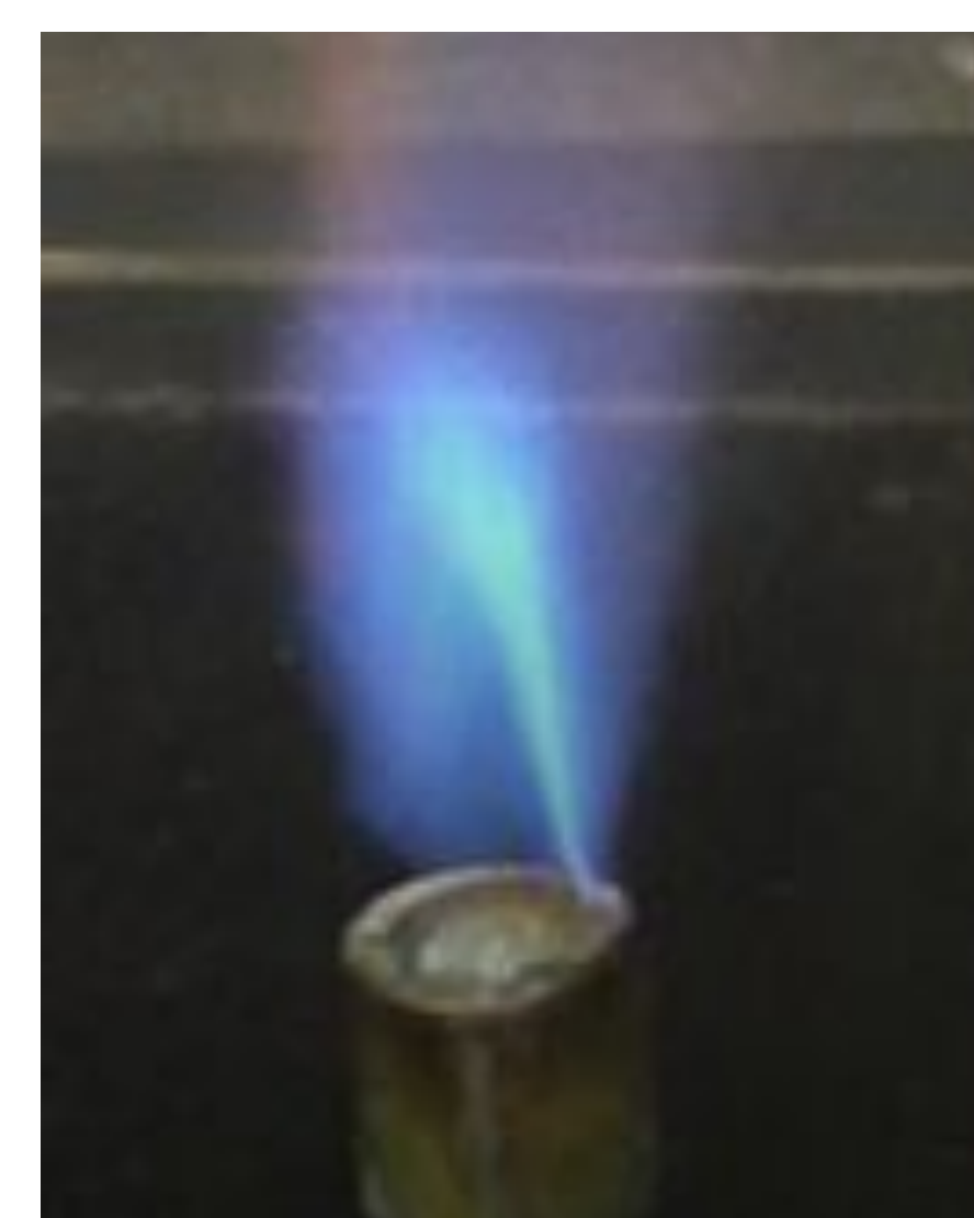
Figure 4: Magnesium chloride flame by spray method
