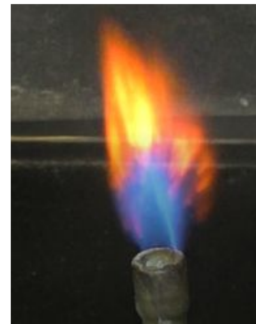
Figure 3: Strontium nitrate flame by spray method
