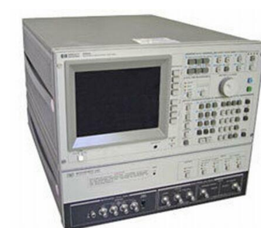
Figure 3: An HP 4194A impedance analyzer
