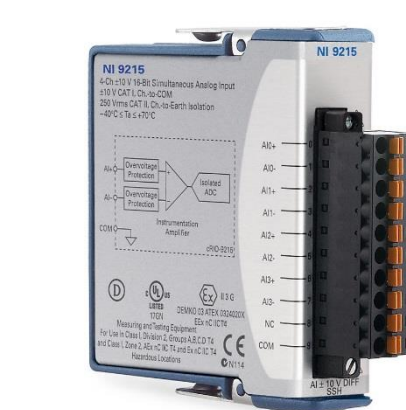
Figure 4: An NI 9215 data acquisition device (DAQ)
