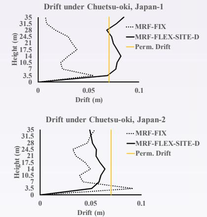
Fig 5. Drift of the structures under Chuetsu-oki, Japan-1 and 2
