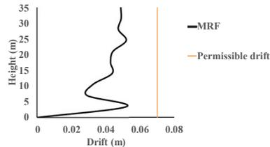
Fig 1. Allowable drift check
