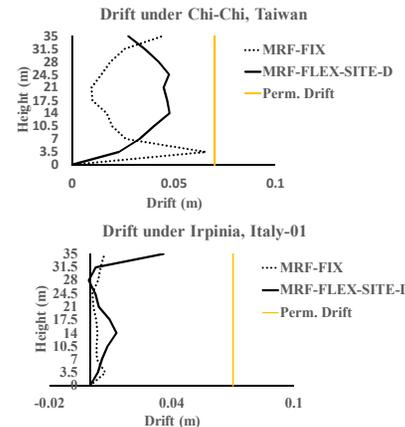
Fig 4. Drift of the structures under Chi-Chi, Taiwan and Irpinia, Italy
