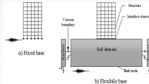
Fig 3. The models of the structures a) fixed base and b) flexible base considering the soil beneath the structure
