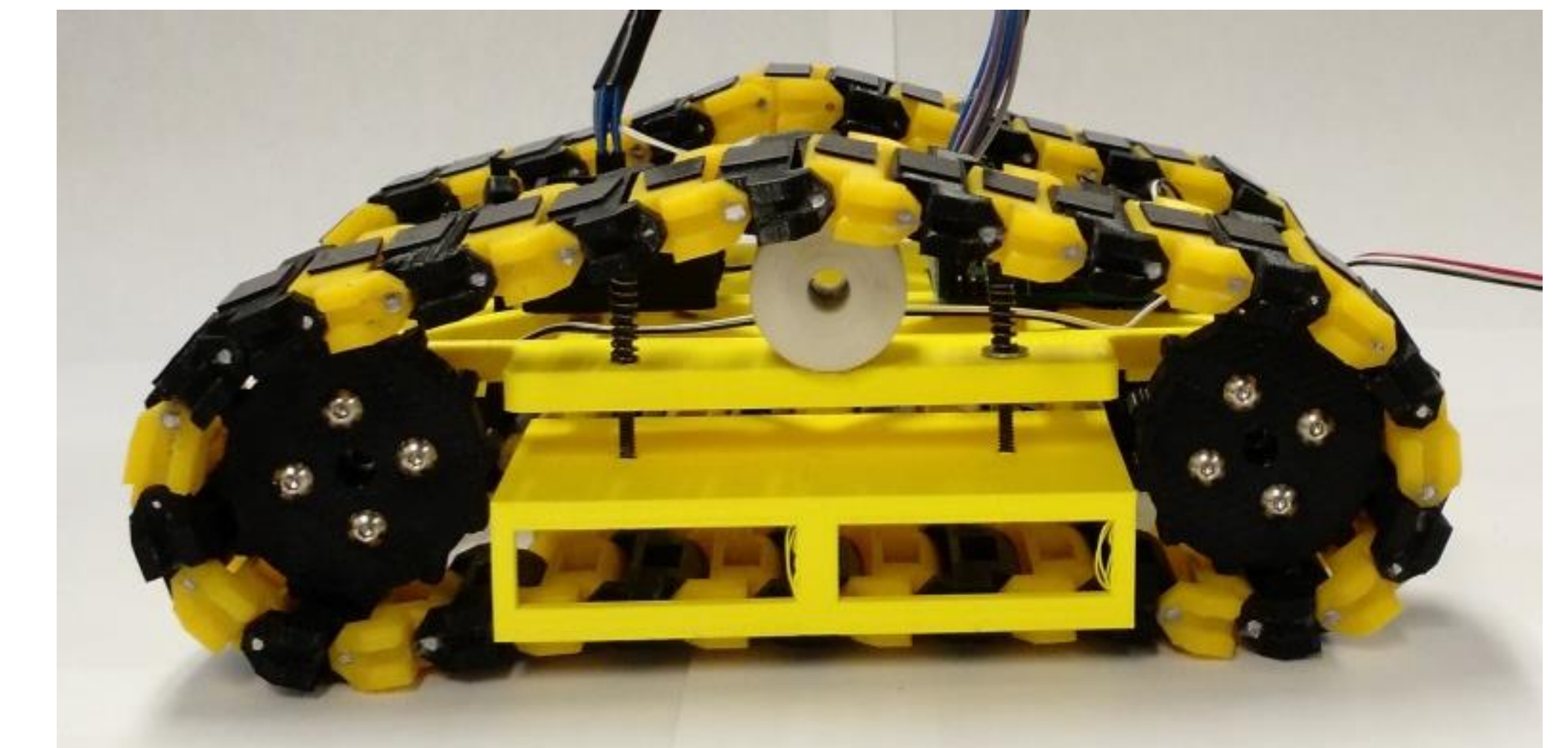
Figure 5: Mobile Robot with Suspension Designed for Suction Cup Tape Dry Adhesive
