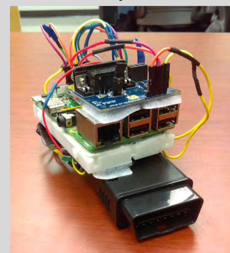
Raspberry Pi CAN Collection device
