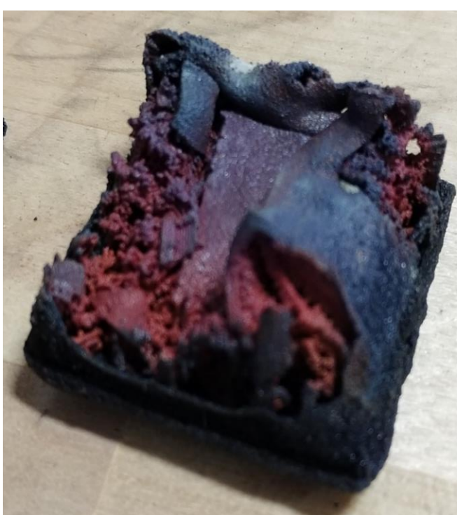
Figure 7. Metal/PLA part collapsed in on itself during sintering due to poor print settings
