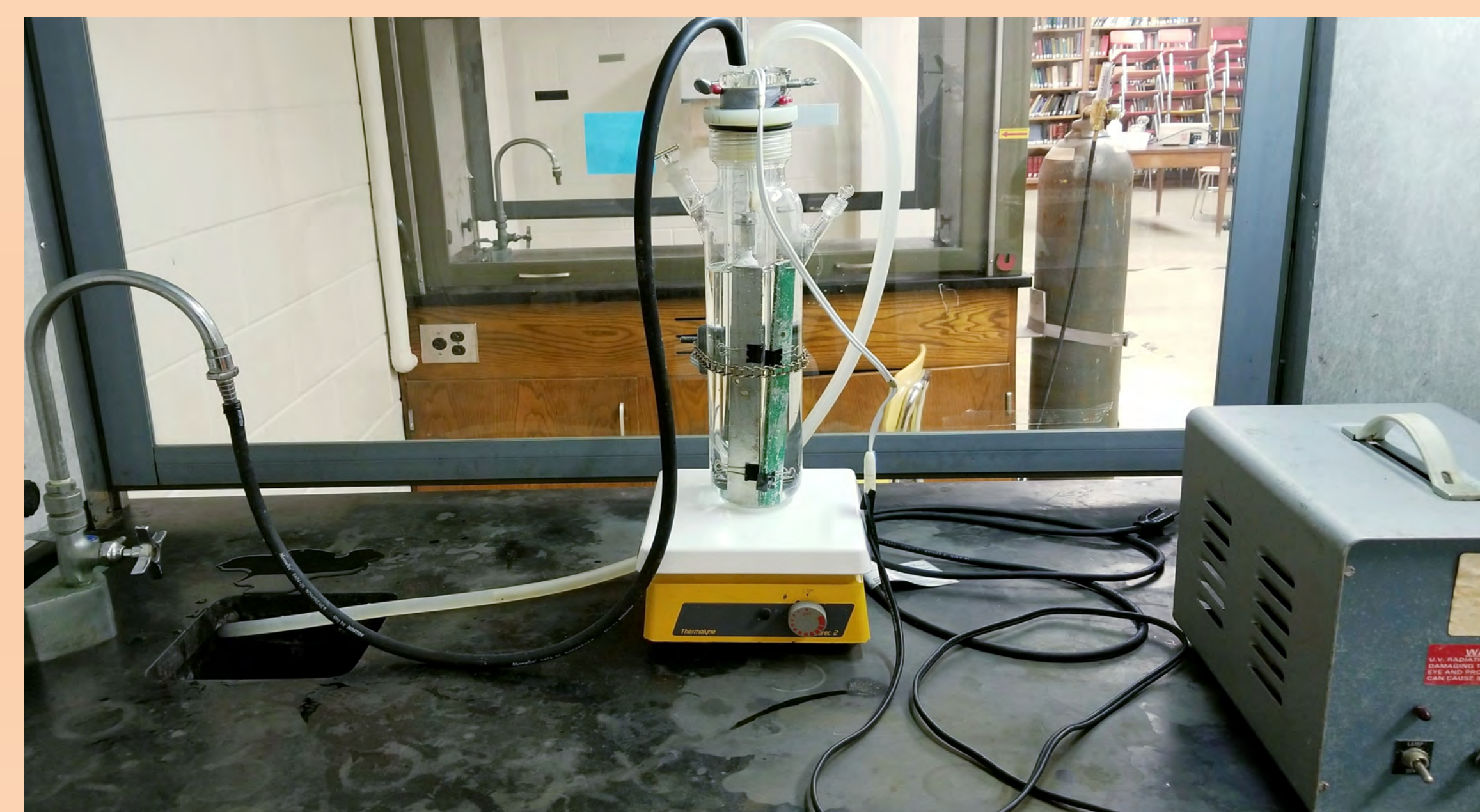
Fig. 5 TiO 2 thin film coating insert on UV Photocatalytic reactor using an aluminum rod.
