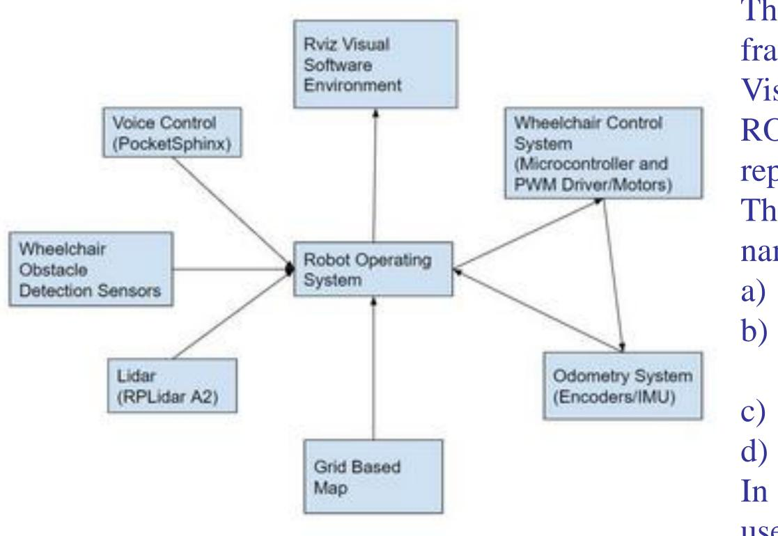
**Mapping:** Mapping is done using a Lidar Sensor, it generates a visual representation that shows all features, obstacles, and objects in the environment
