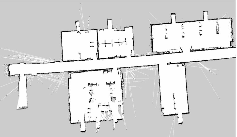
**Figure 1:** Map of the fourth floor of Brown Hall created with a LIDAR Sensor and Hector Mapping Algorithm. Figure 2: Localization of the wheel chair using the AMCL algorithm in the Map created.
