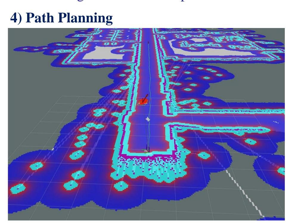
Figure 3: Cost map generated by Lidar and Ultrasonic Sensors, the map generated is used for obstacle detection. Figure 4: The green line indicates the path to be used by the wheelchair to get to its destination, and the red particles with the arrow indicates the actual position/path of the wheelchair
