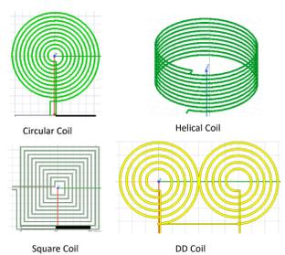
Figure 3: Top performing coils compared [1]
