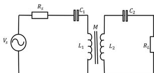
Figure 5: Resonant WPT circuit diagram
