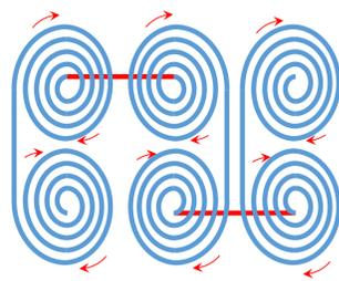
Figure 4: Schematic of Proposed Layered DD coil
