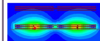
Figure 12: Aluminum Shield on transmitter only
