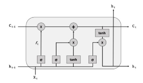
Fig. 1: A Unit Cell of the Long Short Term Memory (LSTM)
