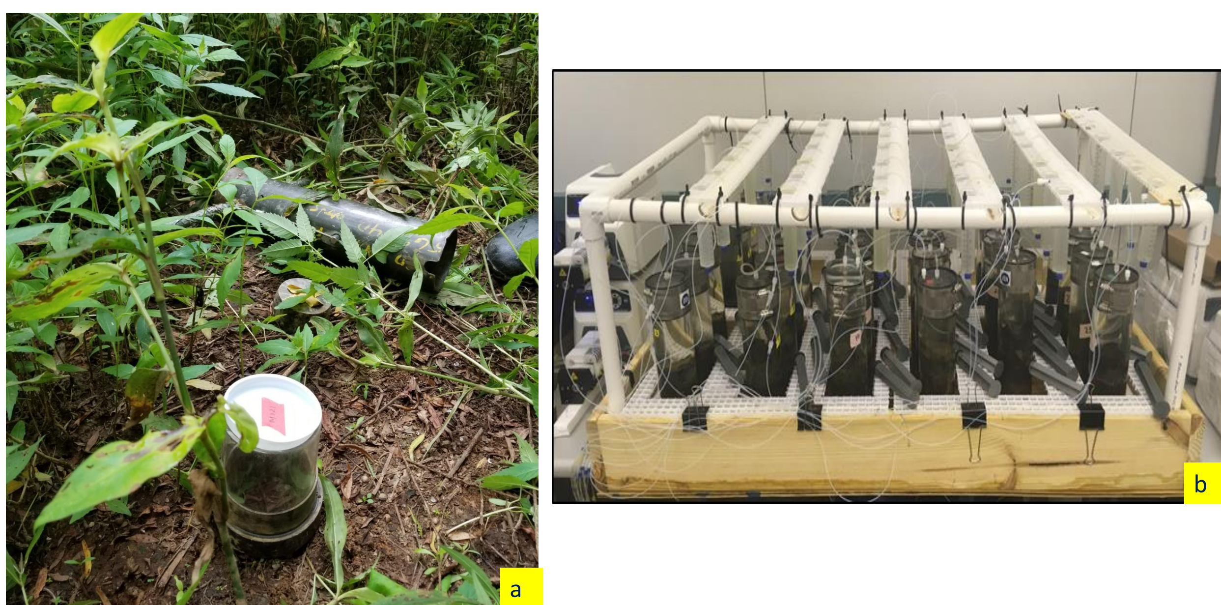
Figure 2. a) Sediment core collection, b) incubation flow through system.
