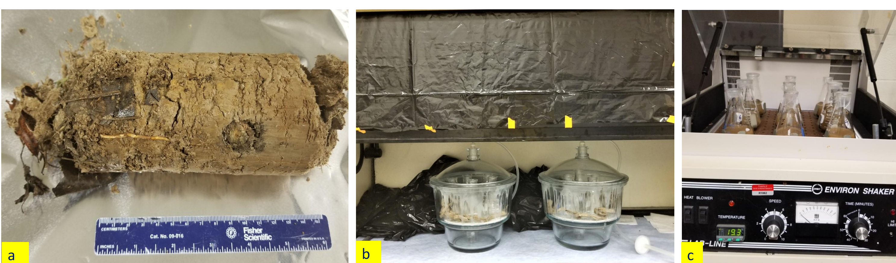
Figure 3. a) A core section, b) chloroform fumigation, and c) samples subjected to shaking for dissolved carbon extraction.
