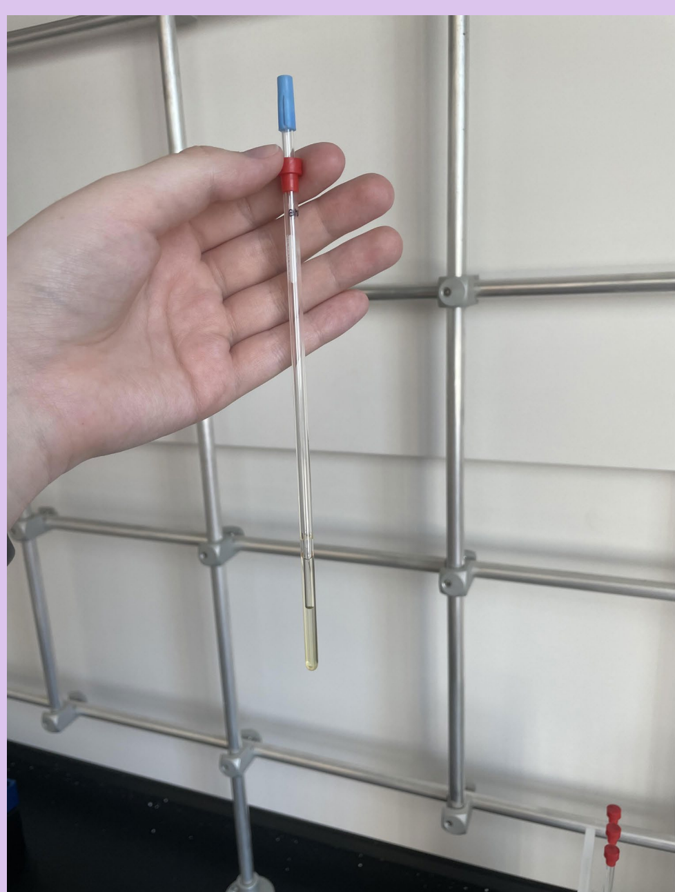
Figure 6.1: EtOH reaction with d-chloroform coaxial tube
