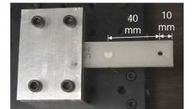
Figure 9: Cantilever beam with 3 mm hole drilled near the free end of the beam.
