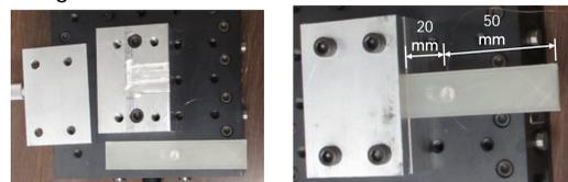
Figure 5: Specimen mounted as a cantilever beam in aluminum fixture
