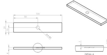
Figure 3: Specimen design and geometric dimensioning (all dimensions in mm)
