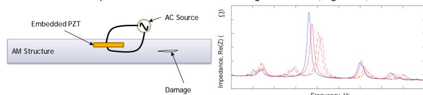
Figure 2: The EMI method being used on an embedded PZT to detect damage in an AM structure
