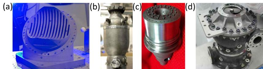
Figure 1. Additive manufactured aerospace components including (a) NASA Pogo-Z engine baffle, (b) SpaceX SuperDraco combustion chamber, (c) NASA's fuel injector, and (d) NASA's fuel pump.
