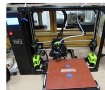
Figure 4: LulzBot TAZ 6 3D printer with printed specimen
