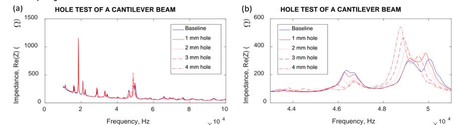
Figure 10: Hole test of cantilever beam specimen with no hole (baseline), 1, 2, 3, and 4 mm (a) broadband measurement from 10 to 100 kHz, measured in 10 kHz segments, (b) 43 to 51 kHz
