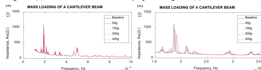
Figure 8: Mass loading of cantilever beam specimen with no mass (baseline), 50, 100, 200, and 400 g (a) broadband measurement from 10 to 100 kHz, measured in 10 kHz segments, (b) 15 to 36 kHz
