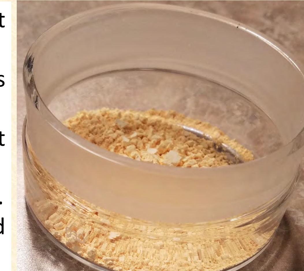
Fig 6: Lab scale synthesized TiO 2 -CdS photocatalyst
