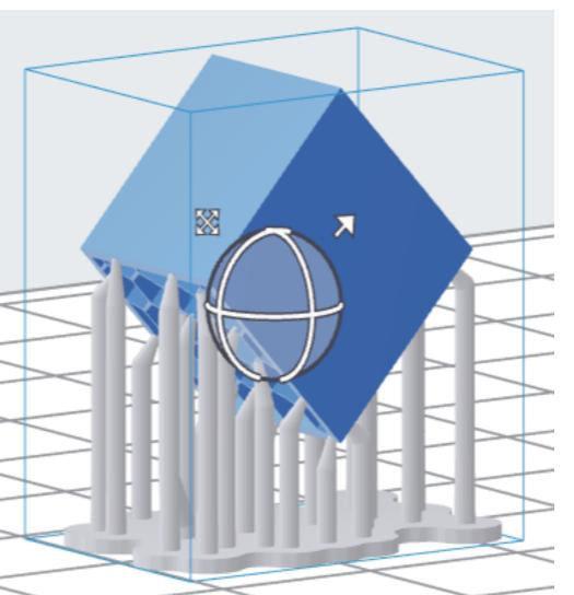
Print Specimen at 20% infill with a hexagonal infill pattern on the PreForm slicing software for SLA printing.
