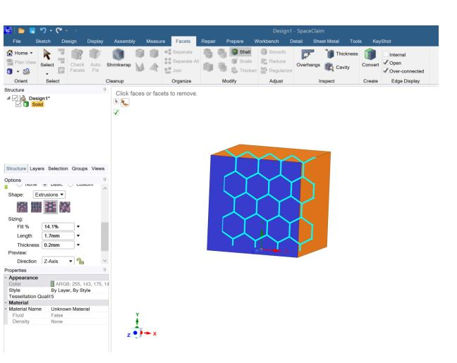
ANSYS SpaceClaim model showing shell and infill generation
