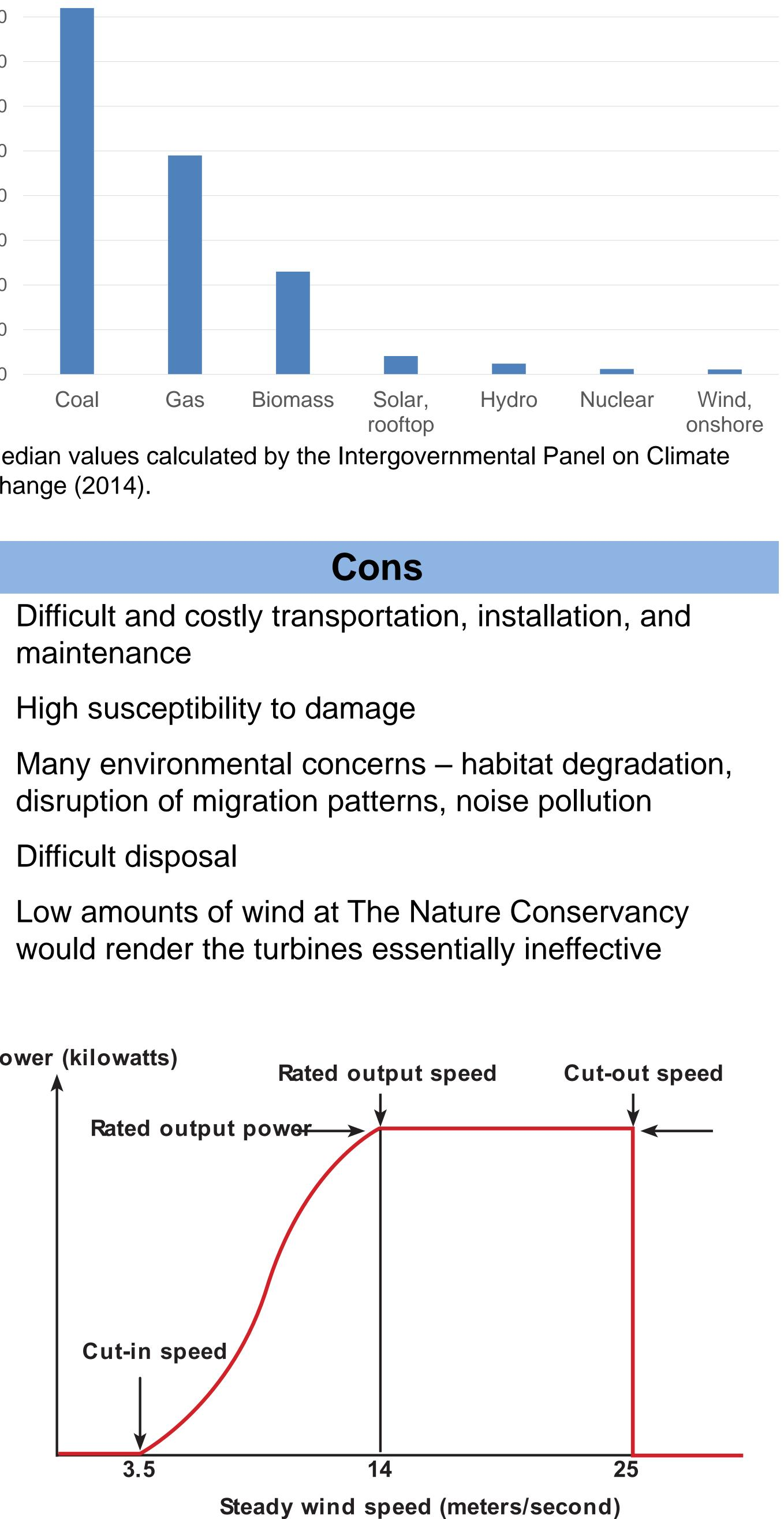
Steady wind speed (meters/second) Typical wind turbine power outlet with steady wind speed.
