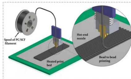
Fig. 1: Layer-by-layer FFF process [2]
