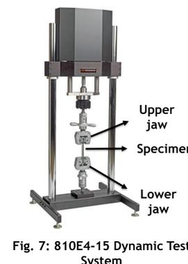
Fig. 7: 810E4-15 Dynamic Test System
