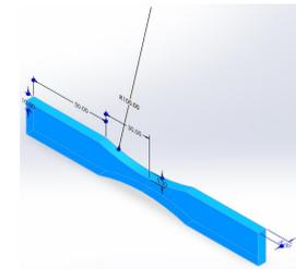
Fig. 3: CAD model of the specimen
