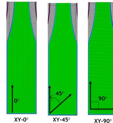
Fig. 5: Filament direction
