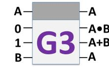
Fig. 5: CRL gate size 4 circuit: AND2 (F1) and OR2 (F7)
