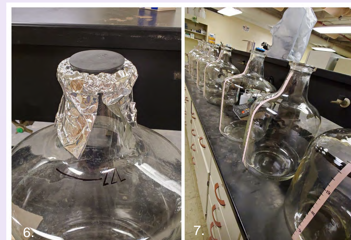
Figure 6. Al foil cap With rubber stopper Figure 7. Cleaned Carboys
