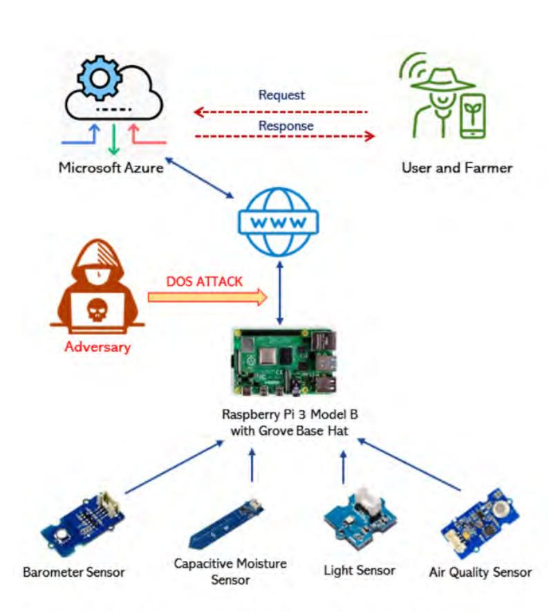
Fig. 3. System Architecture and Attack Surface.
